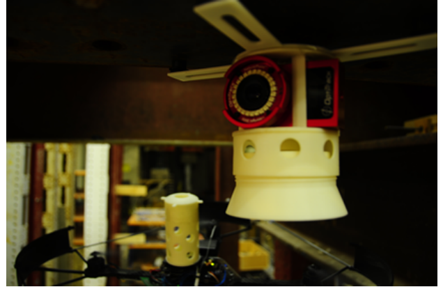
Fig. 1: The passive mechanism in this paper consists of two mating parts that function like a toggle switch to allow a quadrotor to relocate cameras and other small payloads.
